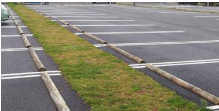
Figure 80: Typical Stormwater storage in a parking lot with drainage through a central filter swale
