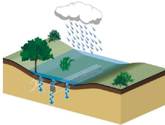
Figure 83: Infiltration swale with a linear infiltration bed at its low point to limit the incidence of puddles and/or increase the storage capacity (Source Architecture & Climat - UCLouvain)
