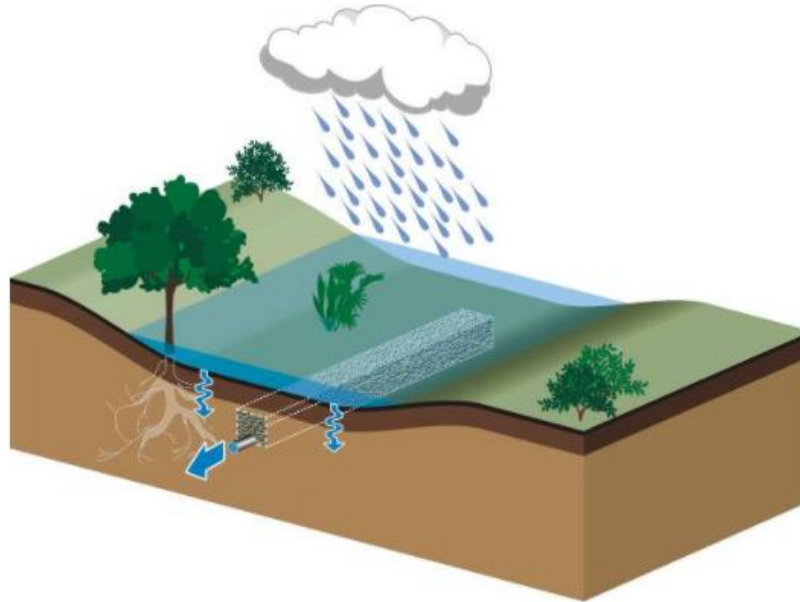
Figure 87: Mixed infiltration and buffering swale, on moderately permeable soil (Source Architecture & Climat - UCLouvain)
