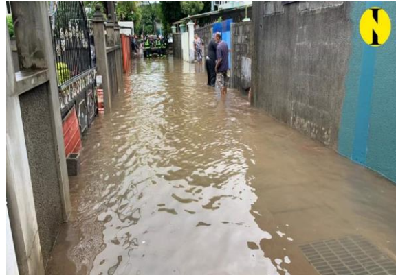
Figure 16: Boundary walls diverting flows along street and to down-slope properties at Chemin Grenier
