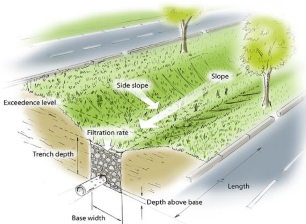
Figure 149: Typical section for swale with French drains beneath (source Innovyze drainage)
