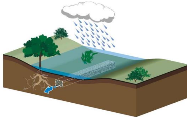
Figure 85: Retention swale on very low permeability soil (Source Architecture & Climat - UCLouvain)
