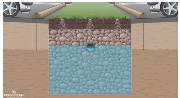
Figure 80: Typical Stormwater storage in a parking lot with drainage through a central filter swale
