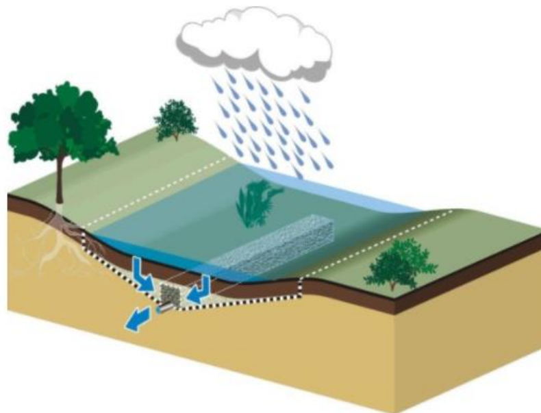
Figure 86: Retention swale with an impervious geo-membrane at the base (Source Architecture & Climat - UCLouvain)
